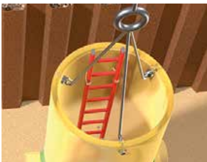
Pic. 2.3 | Manhole shaft, suspended
