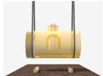
Pic. 2.7 | Lifting an end piece with two straps
