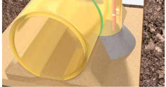
Pic. 3.6 | Concrete filling below the step
