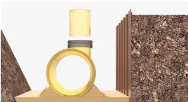
Pic. 3.7 | Installing the entry extension
