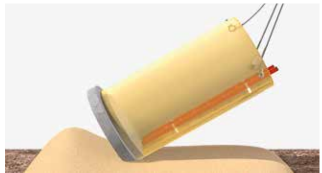
Pic. 2.10 | Raising using suspension gear
