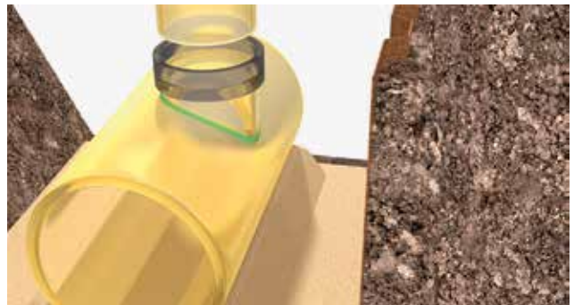
Pic. 3.8 | Installing the entry extension
