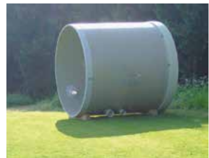
Pic. 2.8 | Storing horizontal manholes
