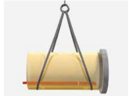
Pic. 2.6 | Lifting a horizontal manhole with two straps
