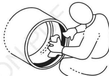
Figure 3-3 Lubrification du joint
